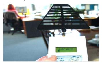
EMR Shielding of adjoining office (just off open plan office on previous page) underneath mobile phone tower. Project carried out by EMR Shielding Solutions using fabric shielding on parti-tion wall and HSF-54 shielding paint on ceiling.
