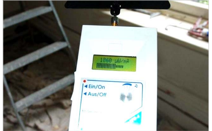
2) Very high EMR reading of 1860 microwatts per metre squared prior to shielding.
