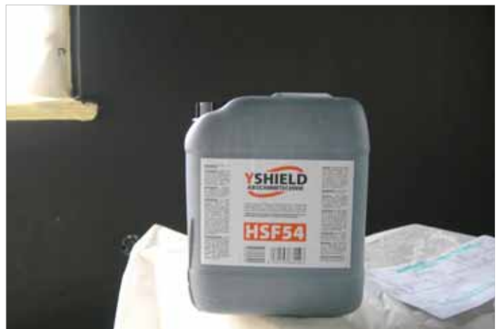
4) They used shielding paint HSF54.
